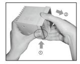
Pressing the front guide of Lock toward ① and squeeze and pull toward ②, it is detached.
