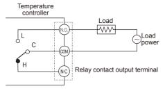
\*\*Be aware that each model has different contact capacity of relay. When load capacity is high, please use sub relay, which has high contact capacity.
