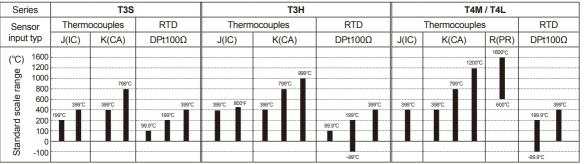
XIn case input sensor is R(PR) type, it is not available to perform correct control under 600°C.
